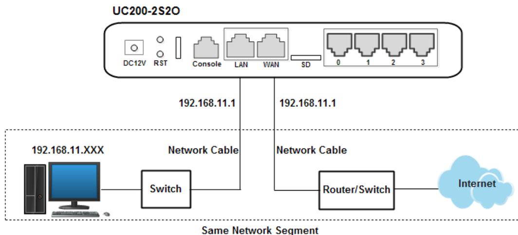
Note: The IP address of PC and that of WAN port of the UC200-2S20 gateway are at the same network segment.
