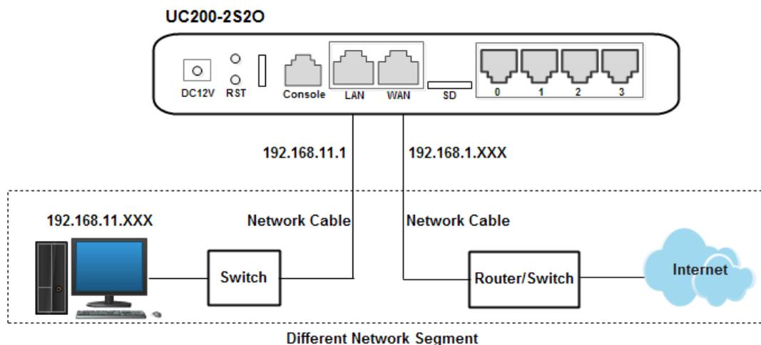
Note: The IP address of LAN port of the gateway and the IP address of PC must be at the same network segment, while that of WAN port is at a different network segment.
