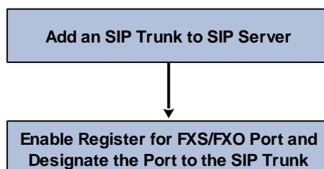
Note: Although 'Register' has been enabled for FXS/FXO port, calls through FXS/FXO port will take inbound and outbound routes as first priority. For outgoing calls, if outbound route cannot be matched, then the registered SIP trunk will be selected. For incoming calls, if inbound route cannot be matched, then the registered FXS/FXO port will be selected.
